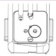
The needle plate is installed with the two holes to the front of the machine as shown. The felting needles will go through the right hole in the front of the felting needle plate
