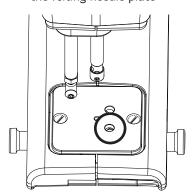
The needle plate is installed with the two larger holes to the right side of the machine as shown. The felting needles will go through the front hole at the right of the felting needle plate.
