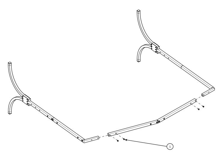
**Step 1:** Lay the two leg assemblies and the top tube assemblies on the floor as shown.
