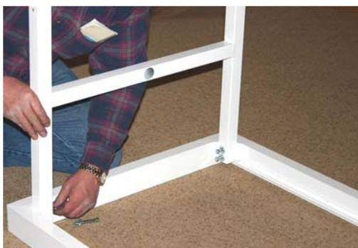
Set the table leg "H" piece inside the table. Using 5/16" x 2 1/2" hex bolt with flat washer, insert bolts (2 per side—4 per leg) **Note:** Leave all bolts loose until all bolts are inserted. Wiggle leg and start all four bolts. If you have trouble starting all four bolts turn the leg around 180 degrees and retry. Tighten by hand as much as possible. Once all bolts are in place, tighten to a snug fit with 1/2" wrench or socket. Do not cross thread or over tighten.
