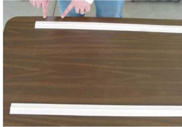
Tape the first track about 1 1/2" from the edge of the table with 2-3 inch wide packing tape. Place tape on the edge of the track, not over the bead on top.
