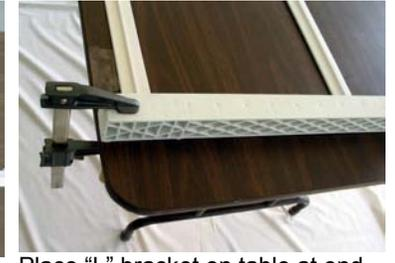
Place "L" bracket on table at end of tracks with the slotted end vertical. The "L" bracket can also be placed over the track if it extends longer. Clamp "L" bracket down tight.
