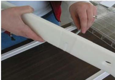
Find the small hole on each of the white side arms. Thread the bolt through the hole. Notice the bolt head goes against the *flat side* of the arm.
