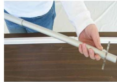
Remove poles with sprockets from box. A large pole is overlapping the small pole. Slide the poles apart to telescope out to the length desired. The poles must overlap *at least* 6 inches to provide adequate strength.
