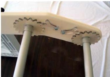
Slide the sprocket pole ends into the holes on the white side arm with Y latches. Hold the Y latches up as you push the pole in so they don't get stuck behind the sprocket.
