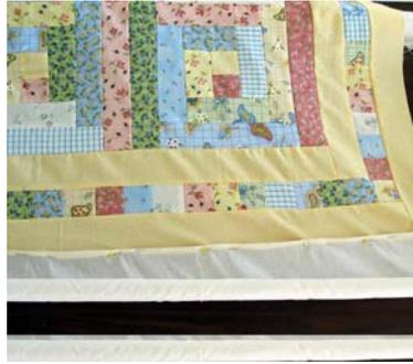
Attach the quilt top to the second (middle) roller by pinning it to the leader. The top is pinned right side up. Place pins close together and close to the edge of the quilt and leader. If fabric is pinned too far from the edge, you lose quilting space. **HINT:** Place entire quilt top over the single take-up roller and roll up completely assuring wrinkles are removed and the quilt top is straight.
