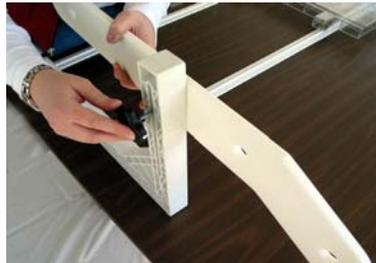
Push the threaded bolt into the vertical guide of the "L" bracket. Thread the black knob on the bolt and tighten. You will adjust the arm up or down with the knob once you get the quilt loaded.
