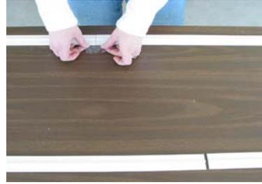
For a smooth ride, stagger the seams of the tracks so you don't get the "sidewalk" effect. Seams should not be directly across from each other.
