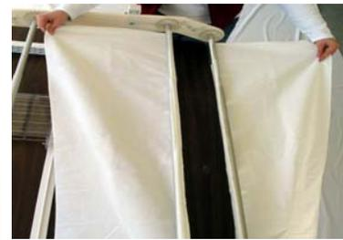
Tape the fabric leaders to the take-up rollers. Notice that these two leaders tape from the inside out. The sprockets only turn one way allowing the leaders to turn from the inside of each take-up roller.
