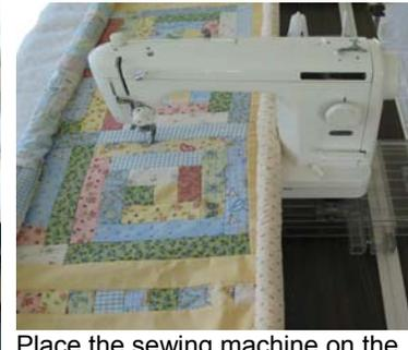
Place the sewing machine on the carriage. Reattach the roller to the sidearm then turn rollers until quilt is taut. Reattach twill tape and begin quilting.
