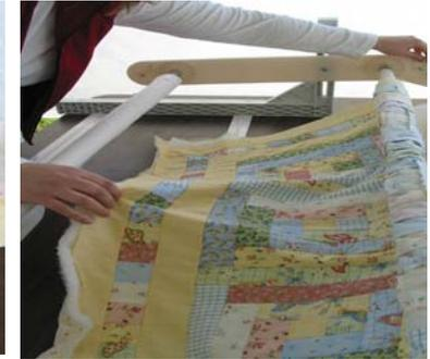
Lift both Y latches to release the sprockets. Pull the quilt backing, batting and top together and pin all three to the take-up roller. (Roller that goes under the sewing machine.)
