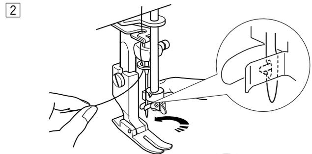
3 Holding the thread with both hands, draw the thread along the thread path ②. Then hook the thread around the guide ③.
