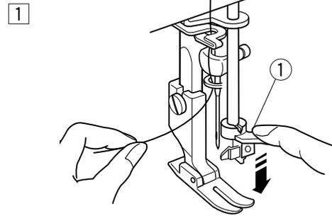
2 Turn the knob ① in the direction of the arrow to insert the hook into the needle eye. The hook ④ comes out through the needle eye as illustrated.
