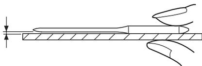
To determine if the needle is defective, place the flat side of needle on something flat (a needle plate, piece of glass, etc.). The gap between the needle and the flat surface should be consistent.
