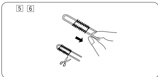
⑤ Remove the fabric from the machine and cut the sewing threads.
