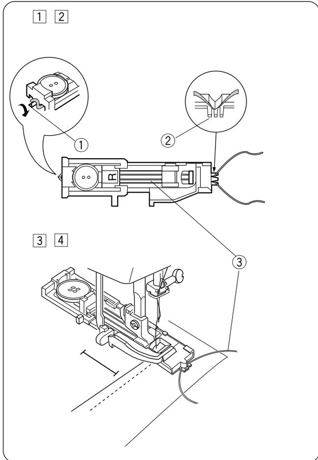
① With the automatic buttonhole foot R raised, hook the filler cord on the spur on the back of the buttonhole foot.
