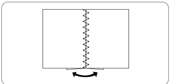
Seam the patchwork pieces with straight stitch and press seam allowance open. Sew pattern #09 on the right side of garment centering over the seam line.
