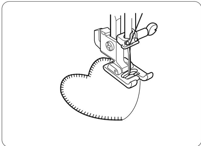
Place the applique on the fabric and baste it in place. Sew, guiding the edge of the applique along the slit on the foot, so that the needle falls off the edge of the applique when it swings to the right.
