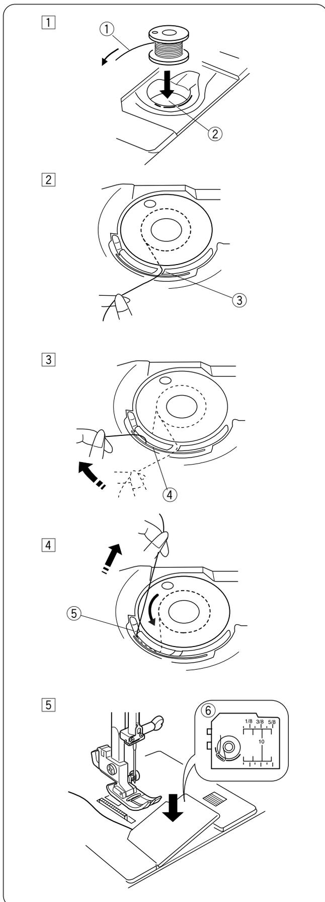
**1** Place the bobbin in the bobbin holder with the thread running off counterclockwise.
