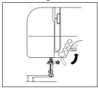
Raise the presser foot. Press the needle up/down button to raise the thread take-up lever to its highest position.
