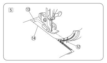
5 Raise and release the foot, and re-attach it with the left side pin. Starting just below zipper bottom stop, sew across the fabric to about 3/8" (1 cm) distance
