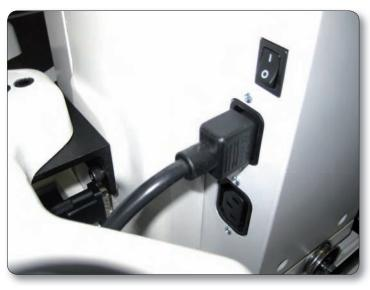
Insert the cord into top power connector on the rear of the machine. Plug the three-prong end into a power source (see Figure 6).
