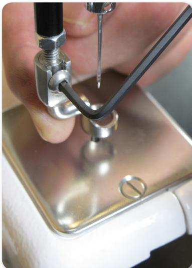
nut; center the foot with the needle; hold the foot in position; and firmly tighten the lock nut (Figure 9).
