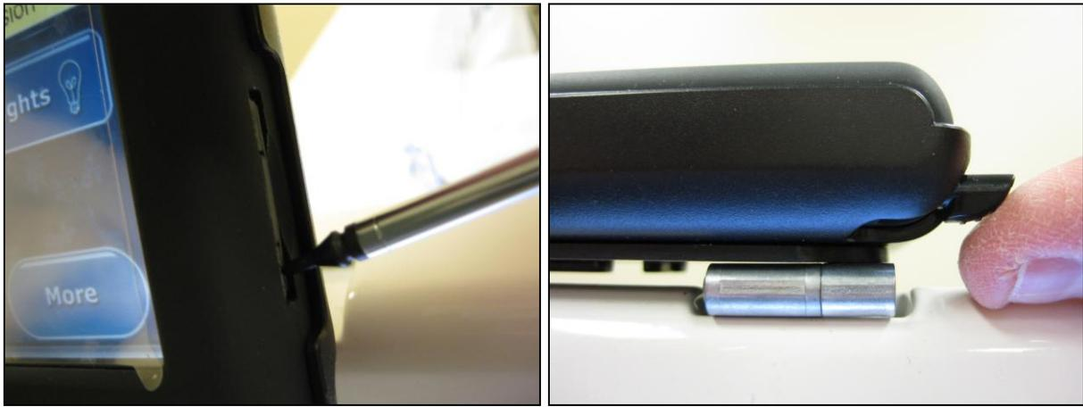
The stylus is stored on the bottom, right-hand corner of the touch screen display. For easiest access to the stylus, tilt the touch-screen display until it is completely flat (screen facing upward).
