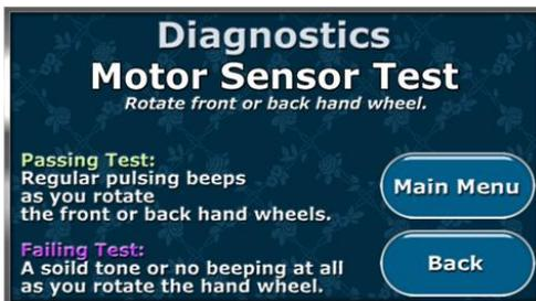
The **Motor Sensor test** can help you determine whether they may be a problem with the HQ Fusion motor. Rotating the front or back hand wheel should result in a pulsing audible “beep.” If you get a constant solid “beep” or no “beep” at all, this indicates a failed test and the machine should be inspected by a qualified Handi Quilter repair technician.
