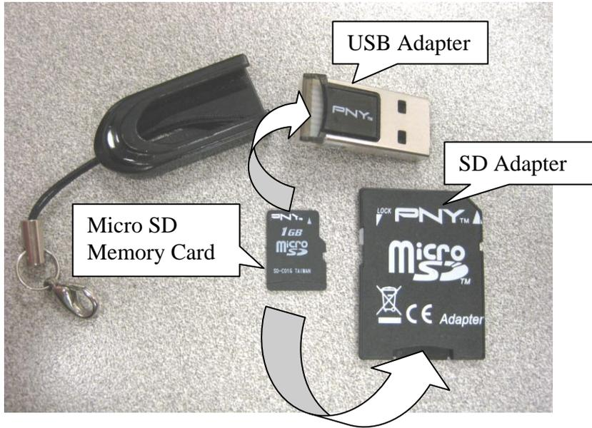
The smallest component (the Micro SD card) is the actual memory device. It can be plugged into the USB adapter to be used on a home computer or the SD adapter to be plugged into the Pro-Stitcher touch screen display.
