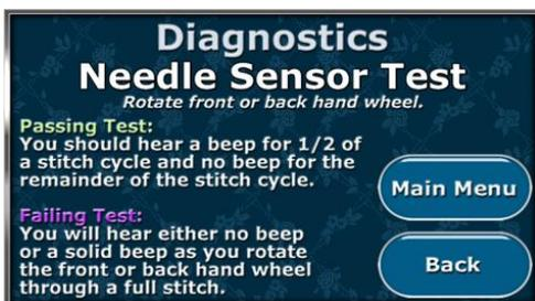
The **Needle Sensor test** will indicate whether the needle position sensor is functioning properly. Rotating the front or back handwheel should result in a “beep” for half of a stitch cycle followed by no “beep” for the other half. If you hear a constant beep or no beep at all for a full 360° rotation of the hand wheel, this indicates a failed test and the machine should be inspected by a qualified Handi Quilter repair technician.
