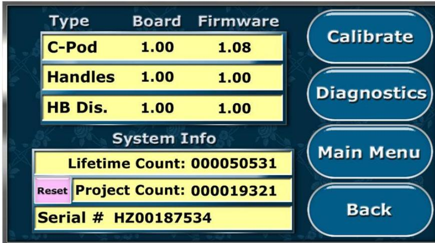
Information contained in the yellow boxes identifies the electronics board revision number as well as the firmware revision number of the HQ Fusion. The serial number of the HQ Fusion is listed at the bottom, just under the Lifetime and Project stitch counters. The Project Counter can be reset to keep track of the number of stitches
