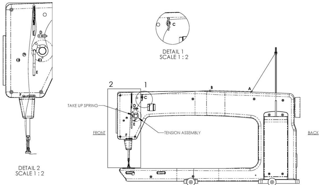
4. Once the thread is in place, be sure that the thread catches on the **take up spring** and then pull it down under the stirrup (thread guide **E**).
