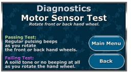
The **Motor Sensor test** can help you determine whether they may be a problem with the HQ Fusion motor. Rotating the front or back hand wheel should result in a pulsing audible "beep." If you get a constant solid "beep" or no "beep" at all, this indicates a failed test and the machine should be inspected by a qualified Handi Quilter repair technician.
