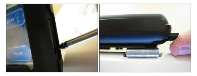
The stylus is stored on the bottom, right-hand corner of the touch screen display. For easiest access to the stylus, tilt the touch-screen display until it is completely flat (screen facing upward).
