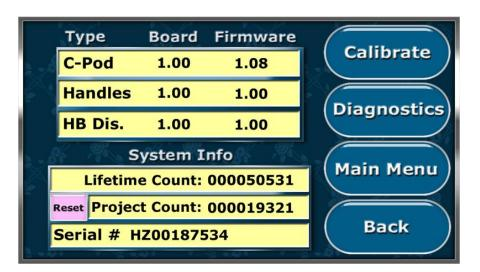
Information contained in the yellow boxes identifies the electronics board revision number as well as the firmware revision number of the HQ Fusion. The serial number of the HQ Fusion is listed at the bottom, just under the Lifetime and Projet stitch counters. The Project Counter can be reset to keep track of the number of stitches
