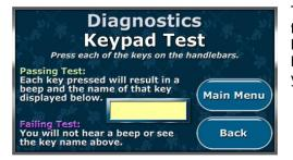
The **Keypad test** allows the user to press any of the four keys on the front or back handles to verify that the HQ Fusion is reading the buttons as they are pressed. When a key is pressed a "beep" will be heard and the name of the key that is pressed will appear in the yellow box.
