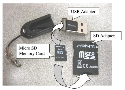
The smallest component (the Micro SD card) is the actual memory device. It can be plugged into the USB adapter to be used on a home computer or the SD adapter to be plugged into the Pro-Stitcher touch screen display.
