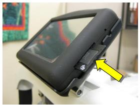
With the update file saved onto the SD card and SD card in place
