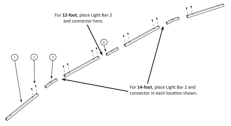
→ Important assembly information for 12-Foot or 14-Foot: Install the Light Bar 2 components (24 inch top tube, one straight connector and four screws) where shown in diagram above.
