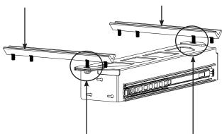
Note: Two longer set screws with nuts replace two short set screws to fix the mounting bracket on the drawer end where the internal table splicers are used. The other screws will not be visible below the internal rivnuts, just the new longer screws for regular nuts.
