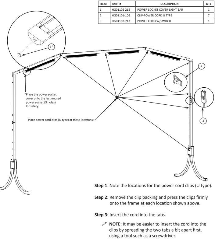
**Step 4:** Place the power socket cover (item 3) in the last unused socket. This will prevent someone from inadvertently placing anything into the socket.
