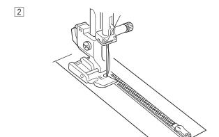
2 Attach the zipper foot E with the pin on the right hand side.
