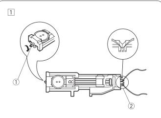
Use the same procedure as the square buttonhole sewing. Set the stitch width to match the thickness of the cord used.
