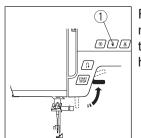
Raise the presser foot. Press the needle up/down button ① to raise the thread take-up lever to its highest position.
