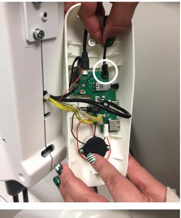
24. Replace the front nose cover being careful of small wires and making sure the two cables now coming out of the coverare located in the notch so they will not be pinched. Do not over tighten the screw into the plastic cover.
