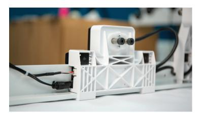
NOTE: The magnet wire length in the HQ Amara/HQ Forte Electromagnetic Channel Lock Kit is different for the two machines. Because the carriage length is shorter for the HQ Amara, customers will need to loop this wire and secure with the provided tie to ensure it is managed properly. This customization will keep the wire away from the underside of the carriage – see image at right.
