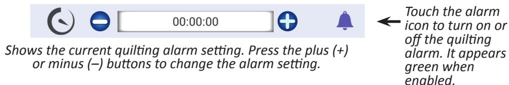
1. Specify the amount of time that will elapse before the alarm will go off. Fine tune the alarm setting by pressing the plus (+) or minus (-) buttons which changes the alarm setting by one minute at a time.
