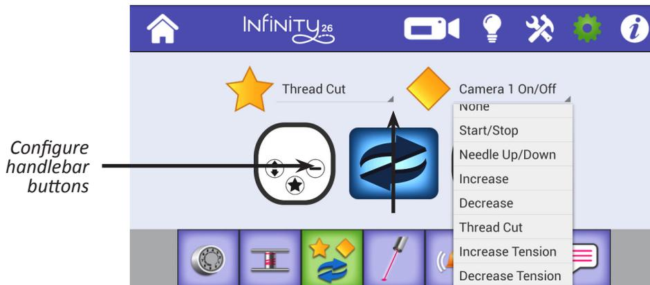
1. Select the down arrow next to the star or diamond to display a drop-down box with the options for the star and diamond buttons.
