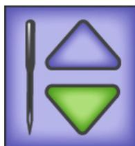
**Needle-stop button:** Touch the button to alternate between having the needle stop in the up or down position when you stop stitching. Your choice displays in green (as shown at the left).
