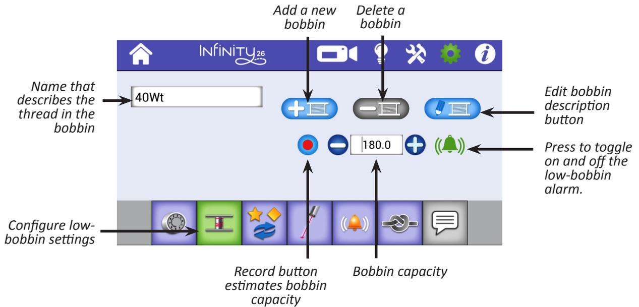
**To add new bobbin configuration and record bobbin capacity**
