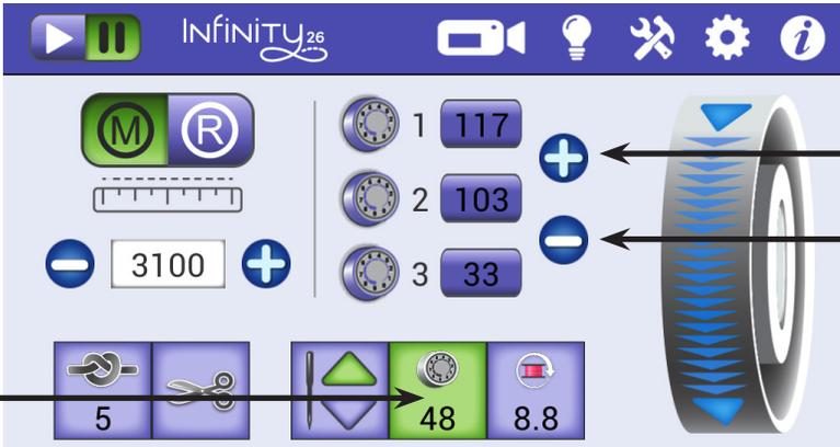
The number on the tension button displays the current tension setting. It changes as you increase or decrease tension.
