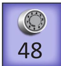
**Easy-Touch Tension™ button:** Touch this button and then use the plus (+) and minus (–) buttons on the screen or on the handlebars to increase or decrease the upper tension. The number on the button indicates the current tension setting.
