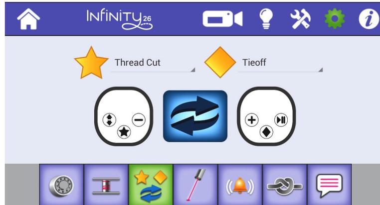
*Press to switch the button configurations to match how you placed the labels on the handlebars. The left button image represents the left handlebar; the right button image represents the right handlebar.*
