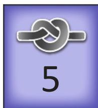
**Tie-off button:** Use this button to perform a tieoff at the start or finish of your stitching. Touch the button and gently move the machine to perform the micro stitches. The number below the image indicates how many micro stitches will be performed.
