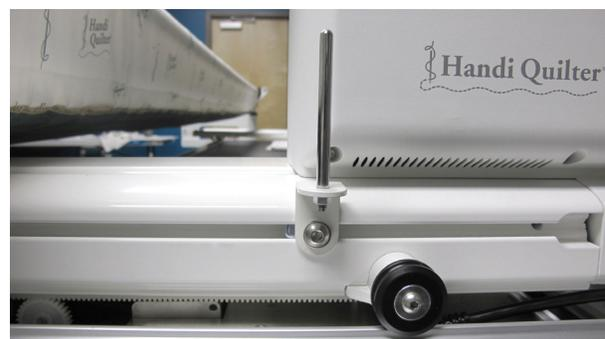
3. Tighten the nut using the 5mm hex wrench. Slide the laser clamp onto the mounting post and tighten the two knobs on opposite sides of the clamp.
