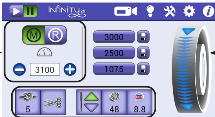
The on-screen hand wheel enables you to rotate the machine's hand wheel from the Main screen rather than reaching around the machine to do it manually.
