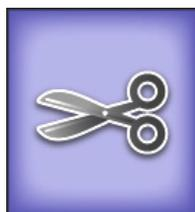
**Bobbin-thread cutter button:** Touch this button to perform a bobbin thread cut. The Infinity cuts the thread at the needle opening in the needle plate, leaving enough bobbin thread for your next pullup.
