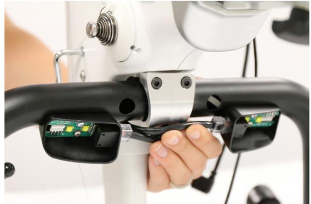
4. Align the bracket and hex screws with the pre-drilled holes behind the machine's head and fully tighten the top two screws with the 4mm hex wrench.
