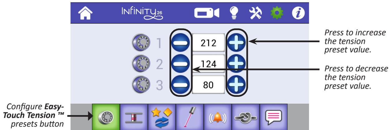
1. Touch the **Settings** icon in the toolbar. Then touch the **Configure Tension Presets** button to open the Tension Presets screen.
