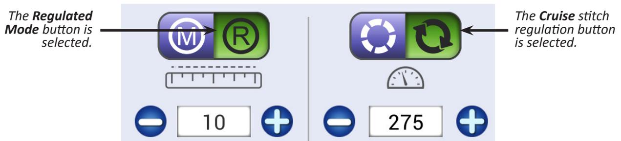
*Shows the current stitches-per-inch setting. Press the plus (+) or minus (-) buttons onscreen or on the handlebars to increase or decrease the setting.*
