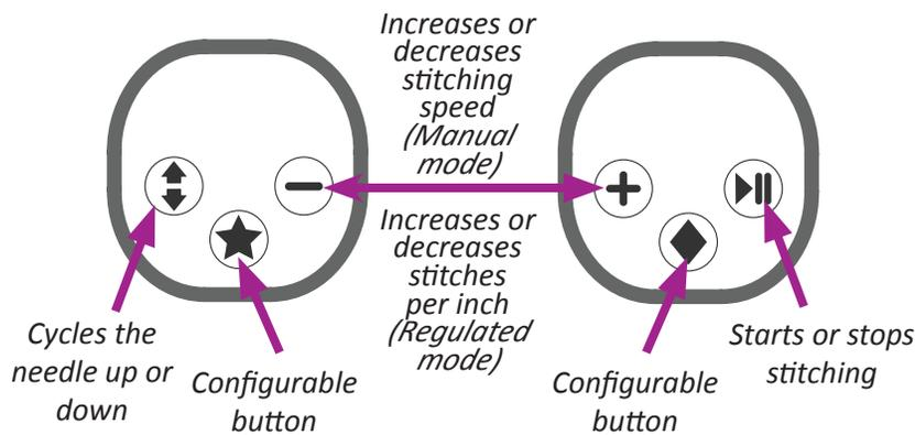
**NOTE:** Pressing the plus or minus buttons on the handlebars also increases or decreases tension after you press the **Easy-Touch Tension™** button on the Main screen. As long as the Easy-Touch Tension button is enabled, pressing the plus or minus buttons controls the tension setting.
