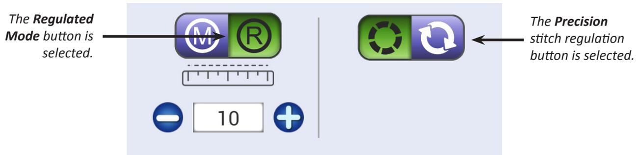
Shows the current stitches-per-inch setting. Press the plus (+) or minus (-) buttons onscreen or on the handlebars to increase or decrease the setting.
