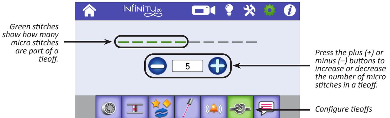
After you indicate how many stitches are in an automatic tieoff, use the Tieoff button on the Main screen to perform the tieoff. Touch the button and gently move the machine to perform the micro stitches.
