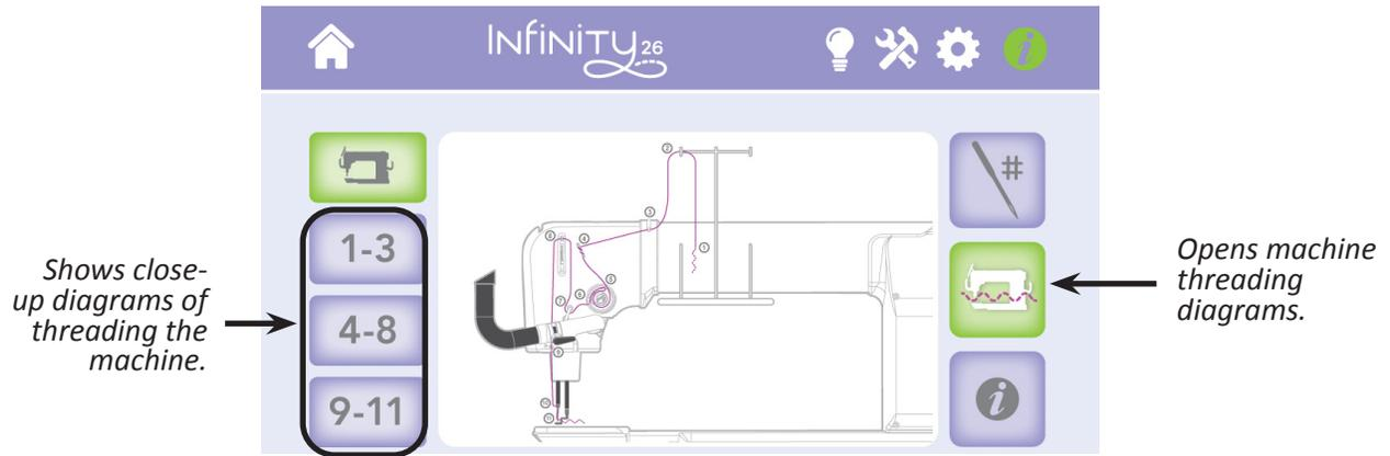
Select one of the buttons along the left to see close-up diagrams of steps 1 through 3, 4 through 8, and 9 through 11.
