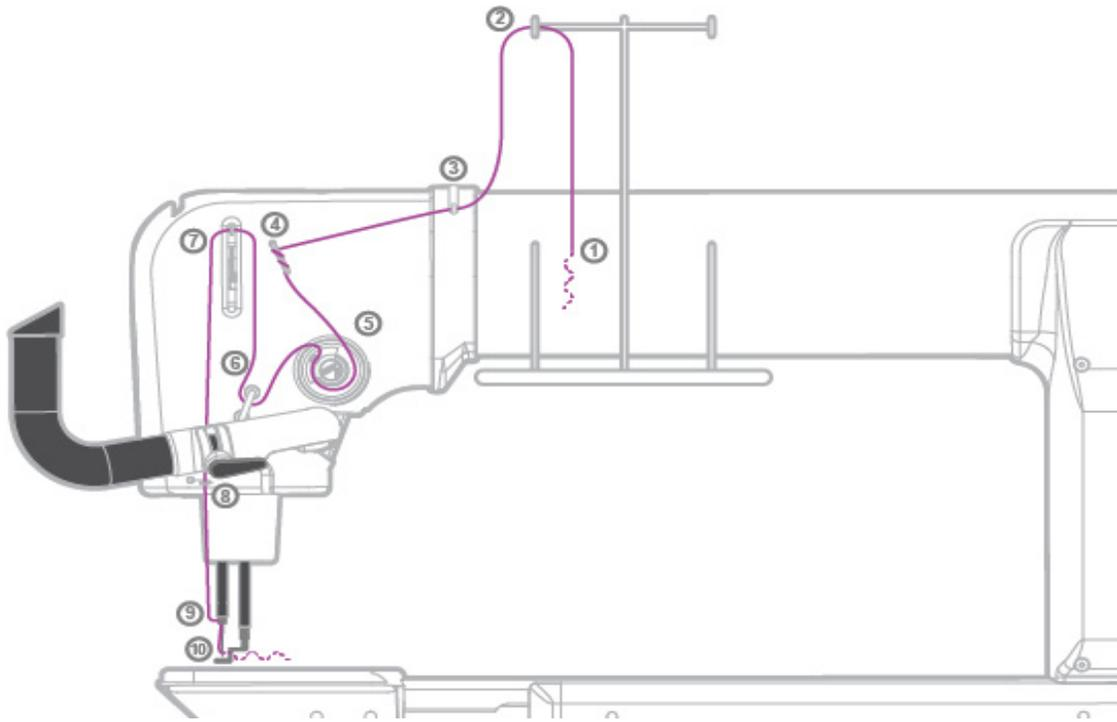
1. Place thread cone onto spool post 2 on the thread tray, insert the thread through the thread-mast eyelet 1 from back to front, continuing to the thread guide 3.
