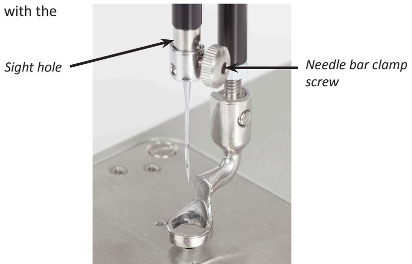
4. Remove the old needle by pulling it down. Discard the old needle in a safe way.
