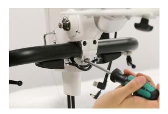
6. Adjust the handlebars forward or backward to a comfortable position for quilting and tighten the bottom screw with the 5mm hex wrench. If using the handlebar lever, fully hand-tighten.
