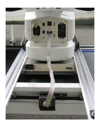
**□ IMPORTANT**: If you ever need to remove the machine from the carriage, disconnect the ribbon cable from the stitch regulator. Failure to unplug the cable when removing the machine from the carriage could result in damage to the cable, encoders, and carriage.
