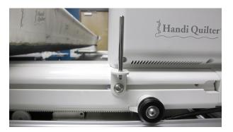
3. Tighten the nut using the 5mm hex wrench. Slide the laser clamp onto the mounting post and tighten the two knobs on opposite sides of the clamp.
