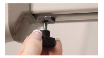
3. Slide the slot of the spool tray onto the knob's bolt. Finger tighten the knob until the spool tray is firm against the throat of the machine.
