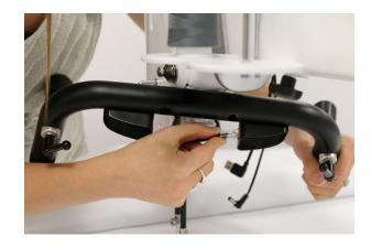
3. Place the 5mm washer on the M5 hex screws and place into the top two holes in the handlebar bracket.
