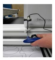
4. Plug the cable end into the laser stylus port on the back of the machine. Wrap the excess cable around the rear handlebars, or insert it into the Handi Accessory Rail and use the T-slot clip to secure.
