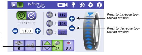
The number on the tension button displays the current tension *setting. It changes* as you increase or decrease tension.
