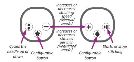
NOTE: Pressing the plus or minus buttons on the handlebars also increases or decreases tension after you press the **Easy-Touch Tension™** button on the Main screen. As long as the East-Touch Tension button is enabled, pressing the plus or minus buttons controls the tension setting.
