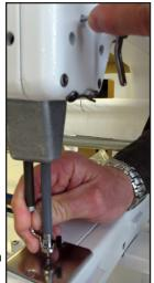
Retighten screw C by turning it clockwise. Tighten the screw enough to hold the foot up, but be careful not to o
