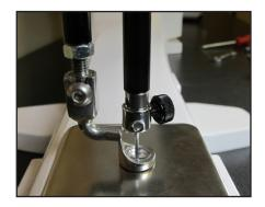
16. Pull down firmly with one finger on the 3mm tool blade while firmly tightening screw C clockwise with the other hand. Pulling down on the tool blade helps ensure that the internal parts engage properly. Remove the business card.
