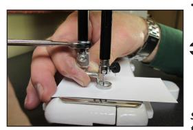
NOTE: Use the lock nut to adjust the foot if it needs to be rotated or the height needs to be adjusted.
