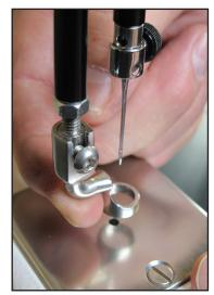
3. Ensure the foot is centered with the needle when the foot is fully tightened with the 2.5mm hex wrench. If it isn't properly centered, loosen the lock nut; center the foot with the needle; hold the foot in position; and firmly tighten the lock nut.
