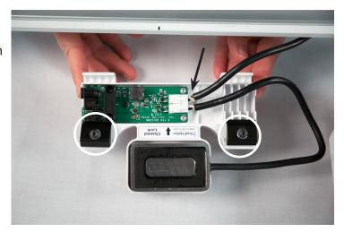
7. Use the zip tie to join the two cables together., and trim off the excess of the zip tie. With the clamps still attached to the Carriage Frame System Y-axis, slide it underneath the carriage. Ensure the clamps are on top of the white rails. (See the next picture.)
