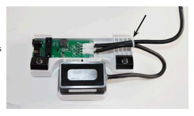
8. Align the arrow with the center measurement mark you made it step 2. Tighten the two screws with 2.5mm hex tool.
