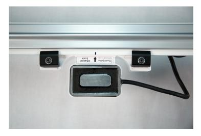
9. Plug the Power Supply Cable and Switch Box Cable into the Carriage Frame System Y-axis.
