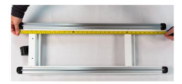
3. Locate Carriage Frame System X-axis. Loosen the two screws with the 2.5 mm hex tool so that the clamps can slide onto the long carriage rails.
