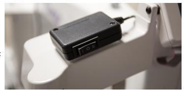
22. Install the Cable Clips and Cable Twist Lock as needed. The Cable Clips enable you to manage the cable to the switch box so it stays out of the way of the machine while quilting. The Cable Twist enables you to manage any slack in the cables. Plug the Power Supply Extension Cord into the Power Supply. Then plug the Power Supply into a power outlet.
