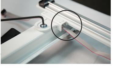
16. Move the carriage to one side of frame. Slide one of the Frame Steel Plates under the carriage toward the frame's sidearms. Align one of the Frame Steel Plates centered under the Carriage Frame System X-axis magnet.
