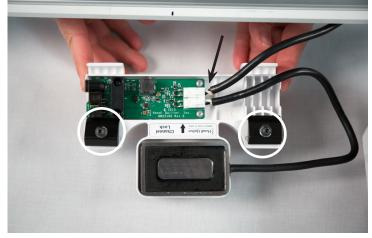
Use the zip tie to join the two cables together., and trim off the excess of the zip tie. With the clamps still attached to the Carriage Frame System Y-axis, slide it underneath the carriage. Ensure the clamps are on top of the white rails. (See the next picture.)
