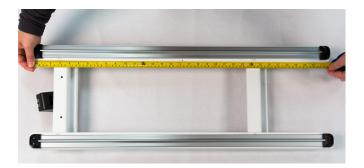
Locate Carriage Frame System X-axis. Loosen the two screws with the 2.5 mm hex tool so that the clamps can slide onto the long carriage rails.
