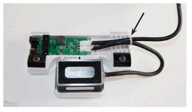
Align the arrow with the center measurement mark you made it step 2. Tighten the two screws with 2.5mm hex tool.
