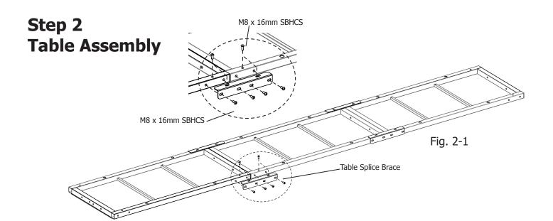
**NOTE:** For this step, a carpeted surface is recommended for the protection of your floor and frame.
