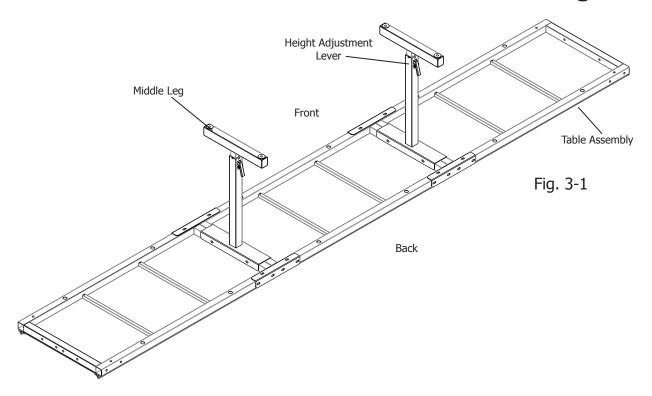
Note: If instructions were carefully followed in Section 2, there should be minimal gap between the table sections where the sections meet. The middle leg/ legs should slide over the two table section end tubes easily. Check to ensure that all table splice brace screws are tightened before tightening the four middle leg screws.
