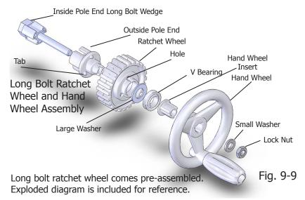
the pole. This will expand the outer pole end, ensuring a tight fit in the pole. Make sure the 3 tabs on the outside pole end, align with the 3 holes in the ratchet wheel, see Fig 9-9. This completes the backing pole.
