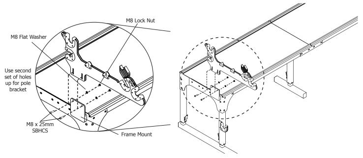
NOTE: If setting frame up with hand wheel on the left side of frame, reverse postition (switch sides) of pole brackets.
