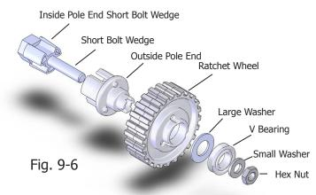
Short-bolt ratchet assembly comes pre-assembled. Exploded diagram is for reference only.
