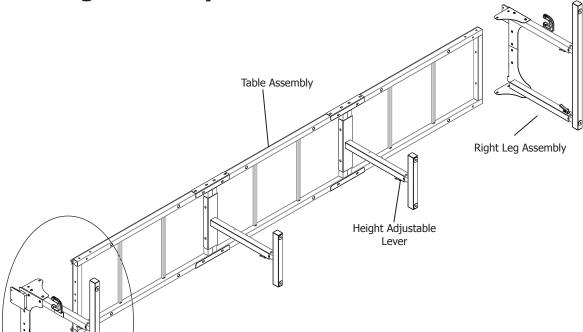
Note: Finger-tighten screws only until all screws are in place, they will be tightened after the table is uprighted once again. See **Step 4-8.**
