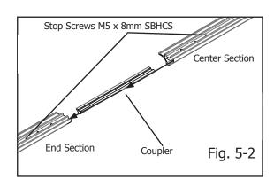
Note: The aluminum track support sections are cut from single sections of extruded aluminum and should align when placed end to end. However, if all directions in Step 5-4 are followed and track supports still do not align properly, try swapping track support sections, so that different ends are joining.
